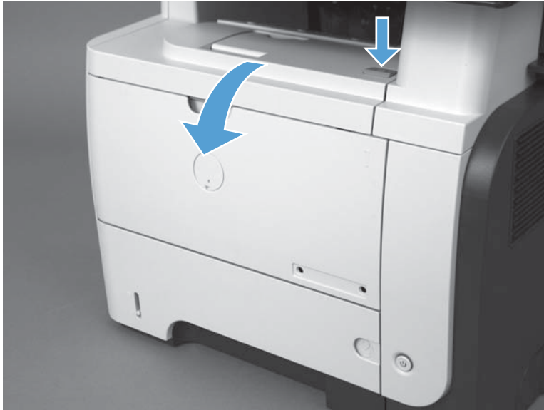
Figure 1-145 Remove the Tray 1 separation pad (1 of 2)
