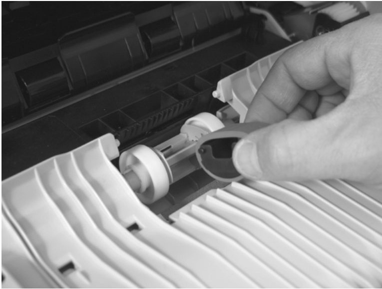
Figure 1-70 Remove the pickup roller (Tray 1; 5 of 5)
