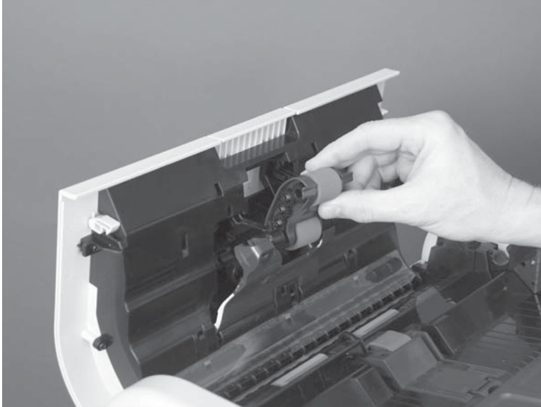
Figure 1-15 Remove the document feeder pickup and feed roller assembly (3 of 3)
