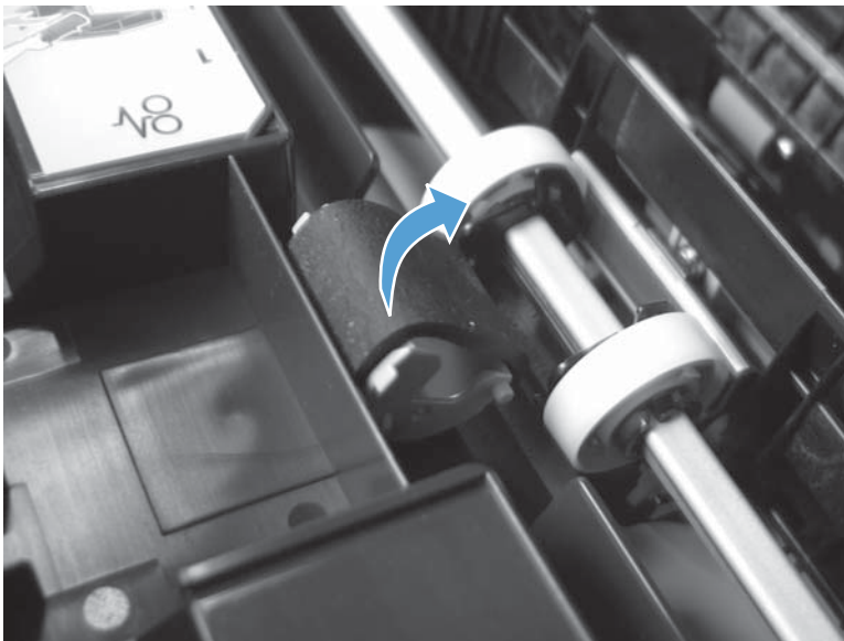
Figure 1-4 Reinstall the Tray 1 (multipurpose tray) pickup roller (2 of 2)
