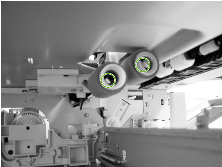
Figure 6-47 Remove the tray 2, 3, or 4 pickup and feed rollers (2 of 2)
