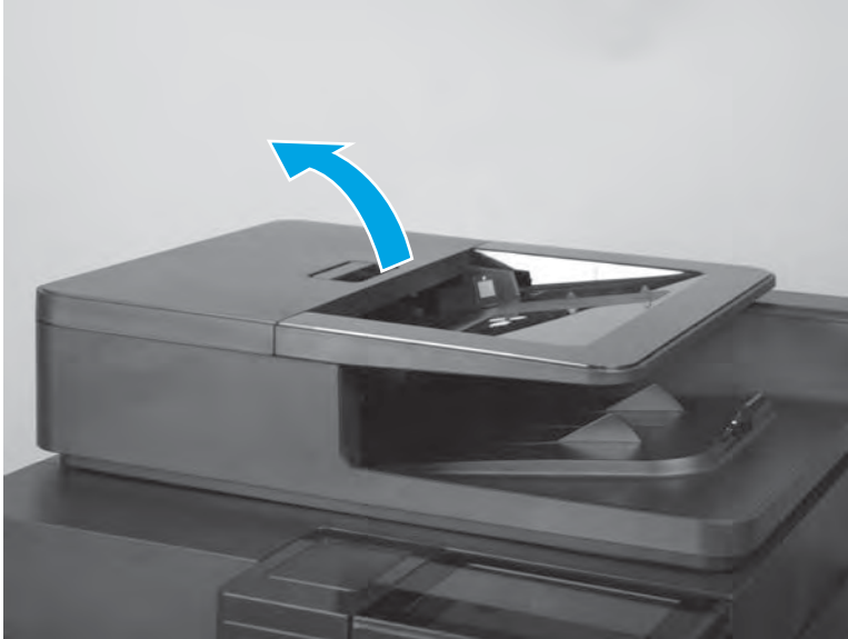
Figure 1-241 Open the document-feeder cover
